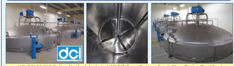
(15) DCI 22,000 Gallon Vertical Jacketed All S/S Cone-Bottom Crystallizer Tanks (Top View)
