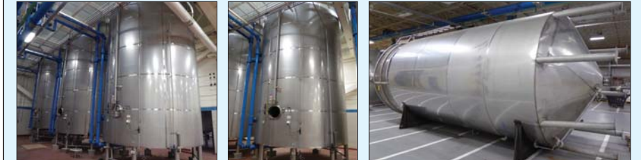
DCI 22,000 Gal. Crystallizer Tanks (Bottom View) - (2) 10,000 Gal. All S/S Dome-Top, Cone-Bottom Tanks
